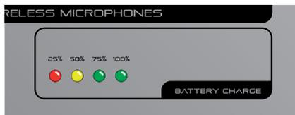
The full charge cycle lasts about 3 hours. For the first charge cycle, however, it would be better that it lasted more than 6 hours. This considerably lengthens battery life.
